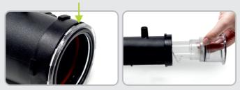
The quartz sleeve can be coated in limescale build up in hard water areas. This should be carefully removed from the quartz sleeve and cleaned with a soft cloth.
