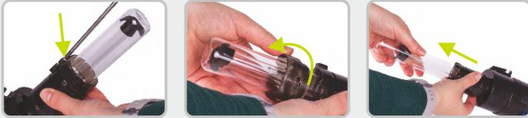
quartz sleeve to access the UV bulb (leave the O-ring located underneath the quartz glass in place).
