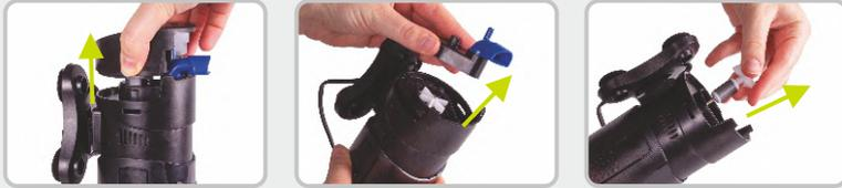
Ensure that the plastic propeller part of the impeller is attached to the magnetic part and that they have not come apart or split. If this is the case you need to replace your impeller. Wash parts with fresh water carefully.
